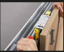
Straightforward height adjustment: the quickest way to adjust sliding doors is when they are closed. Door height is conveniently adjusted from the front and gap alignment can be checked straight away. Alternatively, ceiling height constructions are adjusted from the side.
